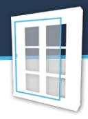
Step 4:• Attach the "L" frame inside of the window box using the included screws.
